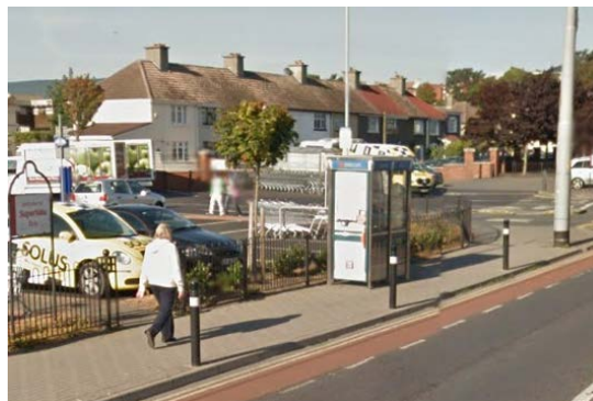
Figure 2 Street furniture reducing footway widths to below minimum (Example drawing sheet 1)
